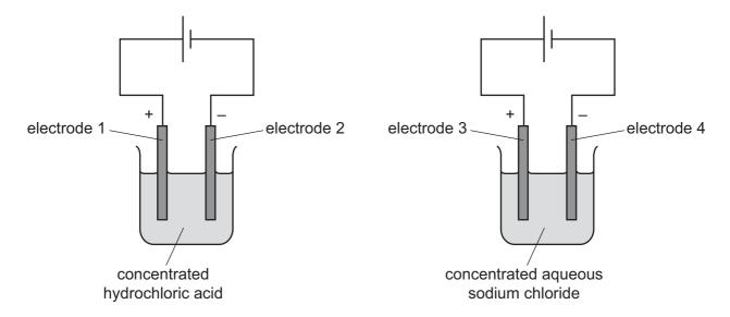
At which electrodes is hydrogen produced?
